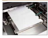
Top and bottom transport belts provide stable transportation of various cover types, and high-precision jog mechanisms register the cover securely for consistent, accurate binding.
