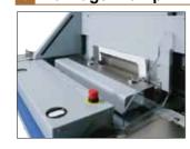
Clamp opening is manually adjusted according to the book block thickness. Rigid clamp mechanism ensures to hold the book block firmly to produce quality book.
