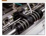
The advanced rotary suction feed system insures fast, smooth feeding of various stock types. Even sensitive stock and digitally imaged covers are fed without any marking.
