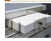
The top-feed cover station accommodates in-line scoring. Up to 70 mm (2.7") of cover stock can be loaded for operator efficiency and longer run length capability.
