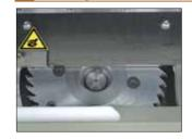
The rotary leveling and notching cutters mill the spine of a book block up to 50 mm (2.0") thick, for optimum glue penetration and adherence.
