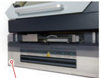
Covers on both sides of knife fold section can be opened.
