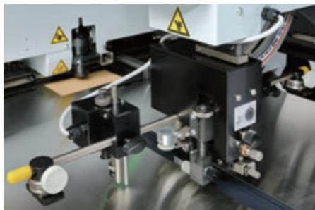
Newly designed suction head and feeding system enables easy setup and consistent feeding. Innovative suction head and assist air\* provide accurate sheet separation and pick-up. Blowing air volume and height of the suction head can be adjusted according to the sheet condition for stable feeding for a wide variety of printed materials.
