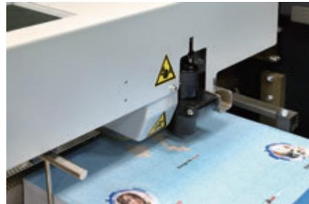
Quality polyurethane rotor provides high speed feeding without scratching. The suction angle adjustment enables stable feeding by adjusting the angle of suction air according to the sheet condition. The supersonic and photoelectric double feed detect sensors come standard for superior double feed protection.
