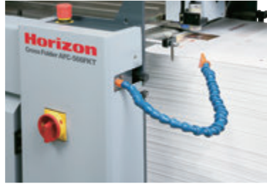
The above photos show the AFC-566F. Left Photo: Side blowing assist air is an option for the AFC-566AKT / 564AKT. Right Photo: Supersonic sensor is an option for the AFC-566AKT / 564AKT.
