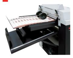
Folded jobs are delivered to the upper conveyor and neatly stacked for easy job handling. Flat creased jobs are delivered to the lower tray.
