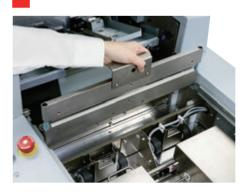
Up to 10 creasing lines can be performed in one pass. Creasing depth can be adjusted. Up and down creasing are performed in one pass. Creasing positions can be adjusted in increments of 0.1 mm / 0.004"
