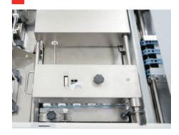
Sheets align to the register guide to ensure straight feeding for accurate creasing and folding. Sheet skew can be adjusted by changing the transport roller pressure on the registration guide.
