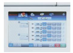
Newly equipped high resolution touchscreen provides intuitive operation. Changeovers including fold pattern, creasing number and up / down crease selection can be done easily at this screen. Up to 200 jobs can be stored in memory for easy recall.
